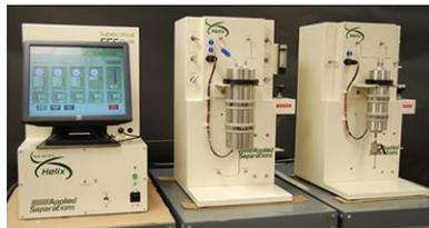
SFE is an alternative technique using supercritical carbon dioxide to extract additives from polymers. It reduces the use, exposure to, and disposal of hazardous solvents, while providing comparable extraction results in less time. This application describes the extraction of Irganox 1076 from polystyrene using supercritical fluid.
